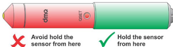
Figure 5: Holding sensor area when the sensor is handheld
